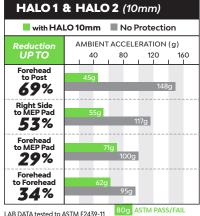
LAB DATA tested to ASTM F2439-11
