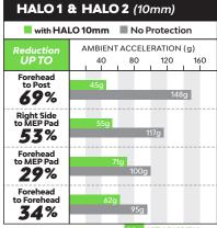
80g ASTM PASS/FAIL LAB DATA tested to ASTM F2439-11
